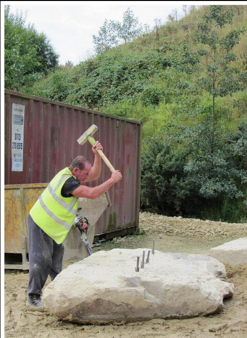
STONE BLOCK BEING SPLIT BY PLUG & FEATHER
