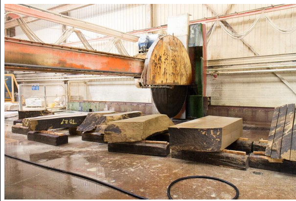
TEN FOOT DIAMETER DIAMOND TIPPED SAW
