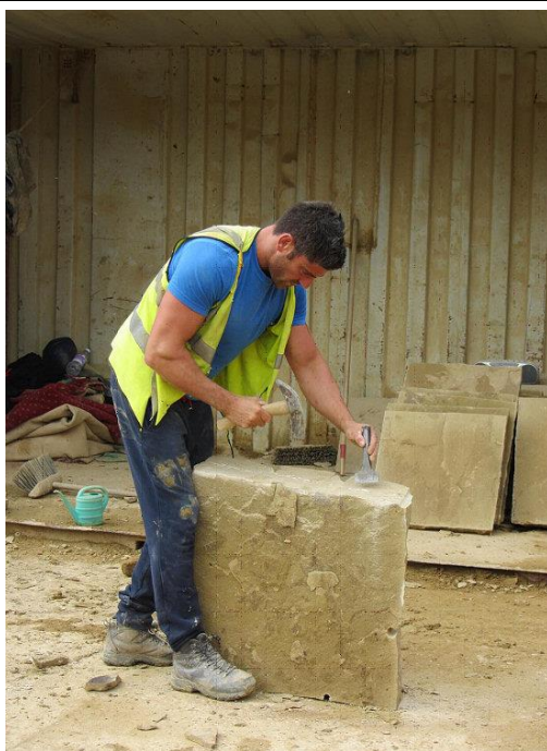
STONE BLOCK BEING SPLIT BY PLUG & FEATHER
